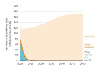
As Figure 6 shows, gas heating equipment sales drop to near zero under this scenario, allowing for the almost complete removal of the gas system by 2050.<sup>35</sup>
