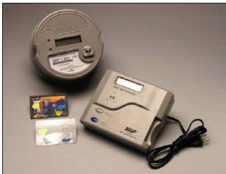
Figure 3-1 M-Power Meter, UDT, and Two Smart Cards
